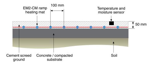
When laying in concrete with a covering of least 25 mm
