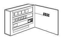
Steel enclosure in wall-mounted construction, equipped with master power switch. Combination(s) 30 mA / C32 A, circuit breaker(s), "On" and "Alarm" warning lights. Completely assembled, cabled ready conneciton and testing. Cable entry points in enclosure floor. Each cabinet is equipped with VIA-DU-20 multi-sensor controller.
