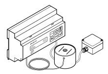
Control unit with combined moisture and temperature sensor and optional ambient temperature sensor.
