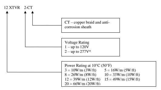
\*The 20XTVR2-CT may also have an alternative maximum voltage of 240V.
