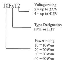
The declared maximum withstand temperatures for the types FMT and FHT are 200°C and 260°C respectively, and the minimum installation temperatures are -40°C and -60°C respectively.
