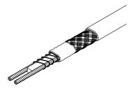
The nVent RAYCHEM XTV range of self-regulating heating cables is used for frost protection of pipes and vessels that require steam cleaning. They can also be used to maintain processes up to 121°C. These heating cables all have fluoropolymer outer jackets offering a high chemical resistance.
