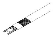
The nVent RAYCHEM KTV range of self-regulating heating cables is mainly used for frost protection of pipes and vessels that require steam cleaning. They can also be used to maintain processes up to 150°C. These heating cables all have fluoropolymer outer jackets offering a high chemical resistance.
