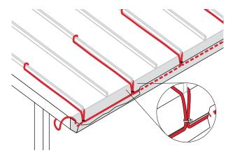
Figure 6: Layout on a standing seam room
