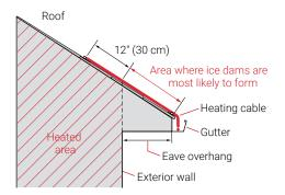
Figure 4: Side view of roof with IceStop system
