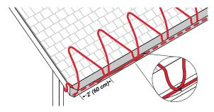
Figure 5: Layout in a zig-zag pattern
