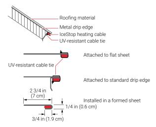
Figure 24: Heated drip edge attachment guidelines
