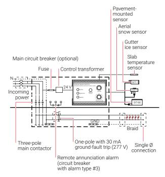
Figure 27: Typical wiring diagram of group control with SMPG1
