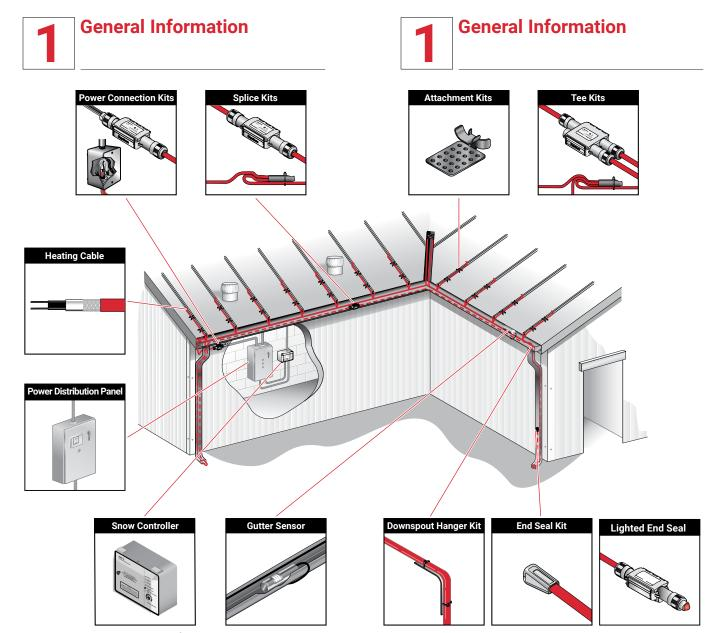
Figure 1: IceStop Roof and Gutter De-Icing System
