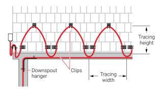
Figure 3: Front view of roof with IceStop system
