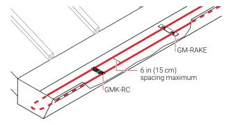
Figure 22: GMK-RC clip on a gutter
