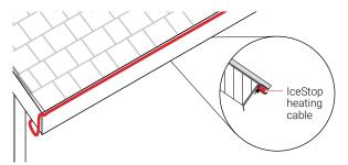
Figure 9: Layout for heated drip edge
