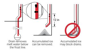
Figure 16: Heating cable at bottom of downspout
