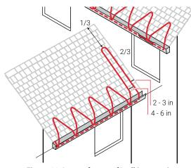
Figure 11: Layout for a roof/wall intersection
