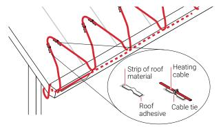
Figure 20: Belt loop approach on a sloped roof
