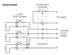
Figure 26: Typical controller wiring-multiple circuits
