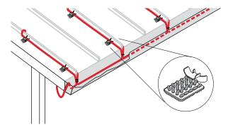
Figure 18: GMK-RC adhesive attachment
