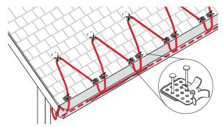
Figure 17: GMK-RC mechanical attachment
