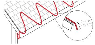
Figure 8: Layout for heated drip loops
