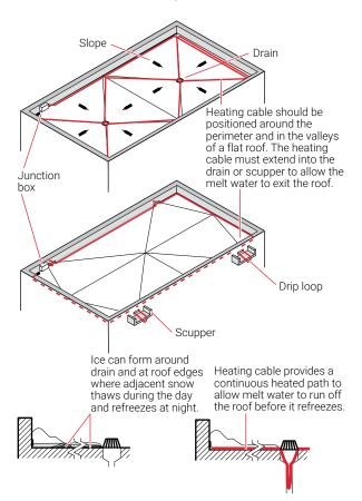
Figure 7: Layout on a flat roof
