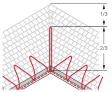
Figure 10: Layout for a roof valley
