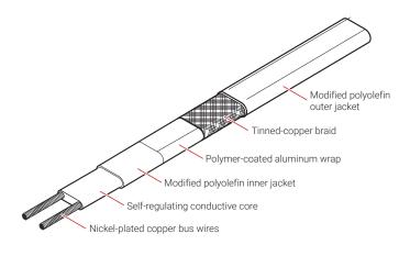
The nVent RAYCHEM HWAT self-regulating heating cables maintain the desired water temperature in a building's hot water distribution pipe network.
