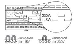
Connect power cable wires to the terminals marked L1 and L2 on the RMM2 module. If power is being daisy chained, be sure to maintain polarity of L1 and L2 wiring for incoming and outgoing wires.
