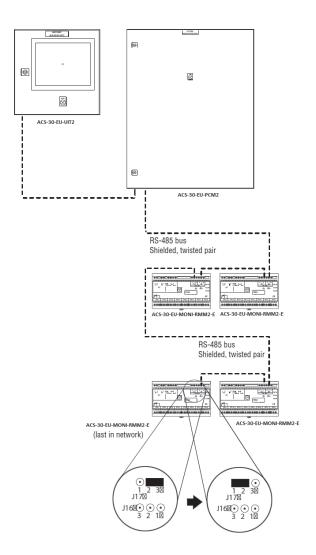
The RMM2 has two sets of terminals for connections to the RS-485 bus. One terminal block allows the RMM2 to connect to the RS-485 bus, the second allows a continuation of the bus to other RMM2 units on the network. Observe polarity, which is indicated on the RMM2.
