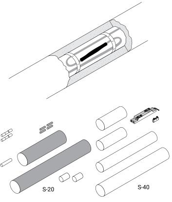
These splice kits are designed for the in-line joining of nVent RAYCHEM selfregulating heating cables.
