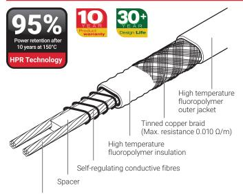
2.3 mm<sup>2</sup> nickel plated copper conductors
