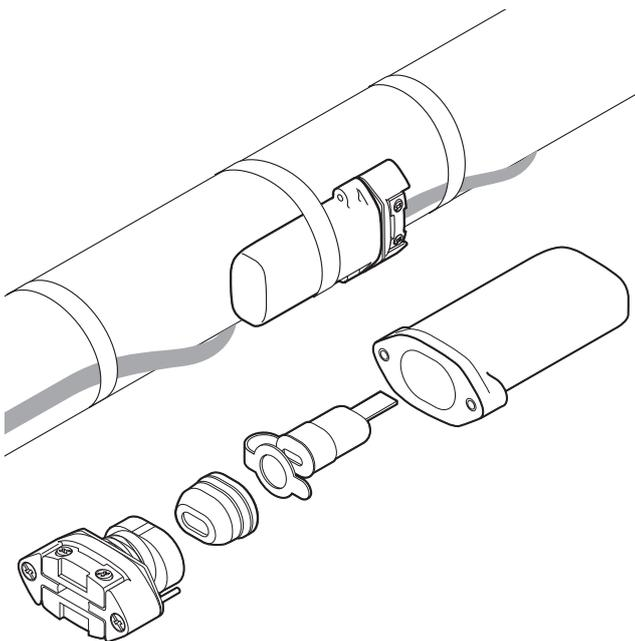
The nVent RAYCHEM E-150 is a cold applied low profile end seal. This universal end seal is designed to fit with all nVent RAYCHEM industrial self-regulating heating cables; BTV, QTVR and XTVR meaning simplified product selection and reduced inventory to stock. It can be used in applications with temperatures ranging from  $-55^{\circ}\text{C}$  to  $+200^{\circ}\text{C}$ . It is approved for use in hazardous areas.
