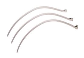
nVent RAYCHEM PBxxx stainless steel straps range are specially designed for holding mineral insulated (MI) heating cables onto pipe. Pliers are the only tool required to pull the pipe strap tight. Buckle and strap avoids over-tensioning of heating cable and eliminates fatigue failures caused by expansion and contraction cycles in operation.
