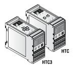
Two versions of this module are available: The NGC-40 Control module for single-phase heaters, NGC-40-HTC; the NGC-40 Control module for threephase heaters, NGC-40-HTC3. Both versions use temperature data to control one single heat-tracing circuit by switching of Electromechanical relays (EMR) or Solid-State Relays (SSR). The NGC-40-HTC/HTC3 also provides ground-fault (leakage) current and line current sensing, monitoring and alarming.
