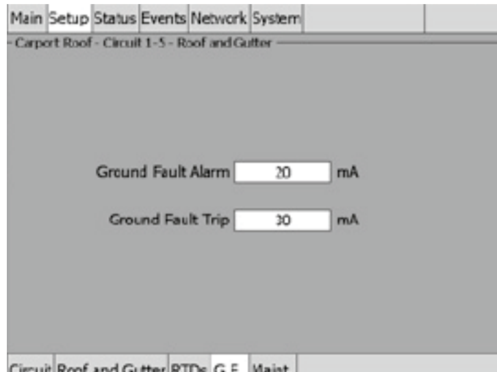
Fig. 3.100 Setup|G.F. Window (Roof & Gutter - Surface Temp Control)
