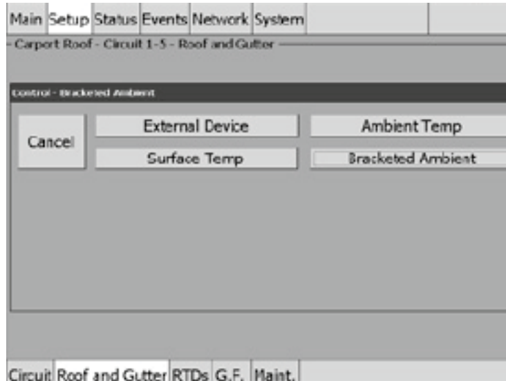
Fig. 3.92 Roof & Gutter - Bracketed Ambient Temperature Control Window
