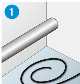
Roll out the trace heating cable. Avoid bending the heating cable beyond the minimum bend radius.
