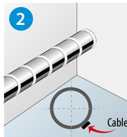
Install the trace heating cable (depending on the thickness of the pipe & the required heating power) along the pipe – in single or multiple runs – and fix it to the pipe at approx. 300mm intervals using the cable ties provided. Ensure the inbuilt thermostat is in contact with the pipe and under the lagging.
