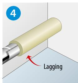
After installation of the trace heating cable, the pipes must be insulated with a minimum of 20mm lagging (Armaflex/PU Foam/Mineral Wool).
