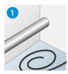
Roll out the trace heating cable. Avoid bending the heatng cable beyond the minimum bend radius.
