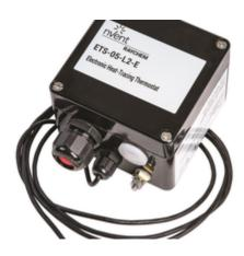
nVent RAYCHEM ETS-05 hazardous area electronic surface sensing thermostats provide accurate temperature control for heating cables. ETS-05-L is adjustable to 199 °C, ETS-05-H up to 499 °C. ETS-05 has a LED to indicate status of the thermostat, heating cable and sensor.
