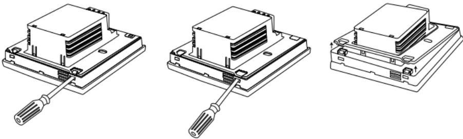
**Step 3:** Screw the metallic support frame to the in-wall box
