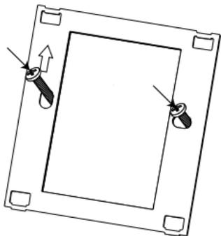
**Step 4:** Install the floor sensor (mandatory for floor sensing mode or room sensing mode with floor temperature limiter). The floor sensor should be installed in a separate flexible conduit all the way to the end, covering the end of the sensor, for easy replacement and to avoid possible signal disturbance on the sensor. For best control performance, position the floor sensor between two heating cables as close as possible to the top floor surface.
