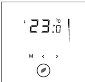
Press the “<” or the “>” to show the set point temperature. It will blink for 5 seconds.
