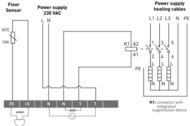
**Connection via contactor - e.g. 3 heating circuits**
