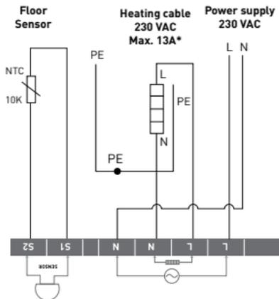
**Direct connection - e.g. single heating circuit**
