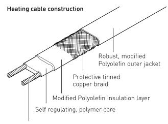
1.2 mm<sup>2</sup> copper conductors
