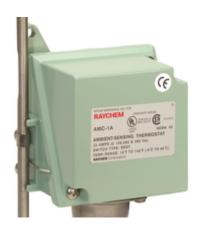
nVent RAYCHEM AMC-1A is an ambient-sensing mechanical thermostat designed to control heat tracing systems for freeze protection applications in non hazardous locations. Used to control a single heat tracing circuit or switch multiple circuits with a contactor, it has an adjustable set point.
