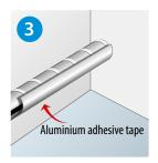
For plastic pipe and plastic components the trace heating cable must be wrapped with an aluminium adhesive tape.
